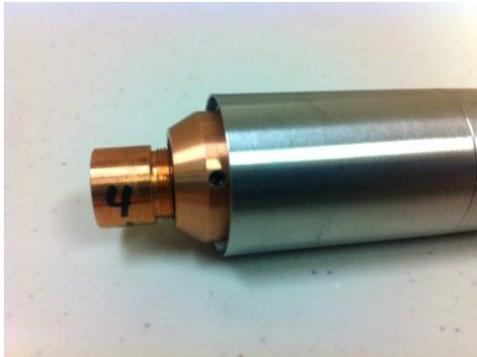
4. Slide the larger diameter end of the heat sink over the exposed diode module on the diode & driver module assembly until fully seated in the heat sink holder and the diode module protrudes beyond the end of the heat sink as shown. **Note:** If called for in your parts bundle instructions, apply the thermal compound to the outer surface of the diode module at this time.
