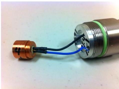
2. **CAUTION:** Remove any static charge on your body by touching a grounded metal object. Thread the separately packaged diode & driver module into the battery compartment until fully seated. **Be careful not to twist or bend the driver leads excessively.** **Note:** If called for in your parts bundle instructions, apply the thermal compound to the "pill" surface at this time.
