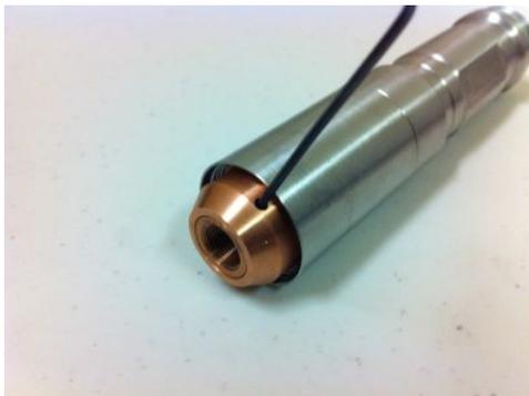
5. Push the diode module into the heat sink until the open end of the module is flush with the end of the heat sink, then tighten the set screw **securely** against the module with the supplied Allen wrench. **Note: If the set screw is not tightened sufficiently, the module could rotate while focusing the lens and break the driver wires or pull them off the diode.** Wipe off any excess thermal compound, if used.
