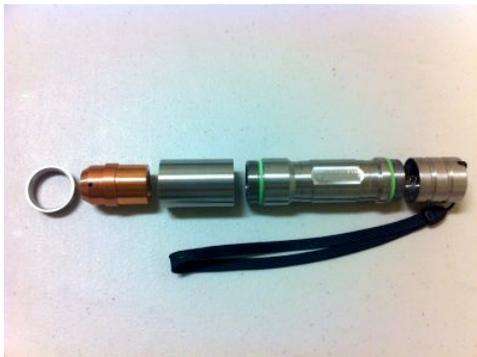
1. Remove the stainless steel laser host assembly from its shipping box and **completely disassemble the host into the five major components shown**. L-R: Bezel/retaining ring, extended and tapered copper heat sink with set screw, heat sink holder, battery compartment, tailcap w/switch & wrist strap.
