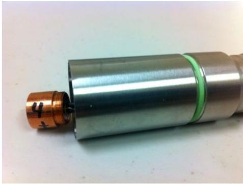
3. Carefully slide the heat sink holder over the diode & driver assembly and thread it onto the battery compartment until fully seated. **Be careful not to twist or bend the driver leads excessively.** There will be some resistance to threading as the battery compartment o-ring is engaged into the heat sink holder during the last two threads.
