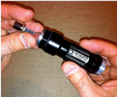
3. **CAUTION:** Remove any static charge on your body by touching a grounded metal object. Thread the diode & driver module into the battery compartment until fully seated. **Be careful not to twist or bend the driver leads excessively.**
