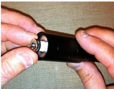
8. Thread the focusing ring/lens assembly about halfway into the diode module. Final focusing adjustment will be completed later. **Reminder:** The **solid slotted end** of the lens assembly faces **away** from the diode. If the lens is installed backwards, the laser dot will have a "bowtie" shape.
