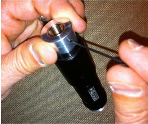
5. Slide the smaller diameter end of the heat sink over the exposed diode module on the diode & driver module assembly until the open end of the module is flush with the larger diameter end of the heat sink, then tighten the set screw **securely** against the module with the supplied Allen wrench. **Note:** If the set screw is not tightened sufficiently, the module could rotate while focusing the lens and break the driver wires or pull them off the diode.
