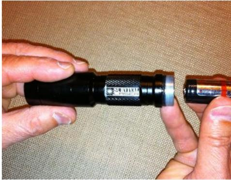
9. **WARNING:** Beginning at this step **put on your protective laser safety goggles** and ensure that anyone in the vicinity of your laser is wearing appropriate laser safety goggles. You must assume that your laser will begin functioning as soon as you screw on the tailcap. Install the charged batteries, **positive end first**, into the battery compartment.
