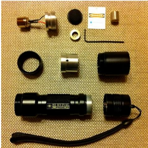
2. Remove and unpack all parts from the laser parts bundle and **completely disassemble the laser host into the five major components shown**. Verify that all parts are included in the bundle. **L-R:** diode & driver module, lens cap, lens focusing ring, laser warning label, 0.050" Allen wrench, AR coated acrylic lens assembly, bezel/retaining ring, heat sink w/set screw, heat sink holder, battery compartment, tailcap w/switch and wrist strap.
