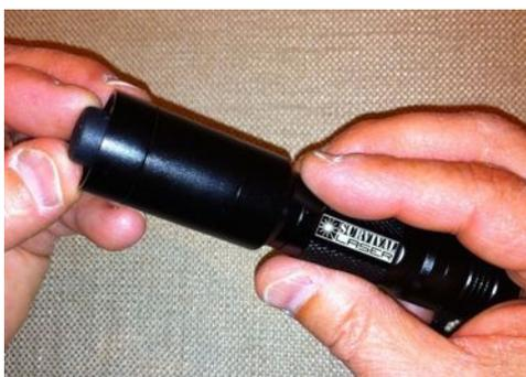
12. Place the lens cap over the lens when your laser is not in use. **CAUTION: Never** operate the laser with the lens cap in place. The cap may burn and combustion residue may be deposited onto the lens surface that can be extremely difficult to remove. **IMPORTANT: DO NOT** disassemble the laser once it is assembled. Doing so may break the wires connecting the driver to the diode and will invalidate your warranty.
