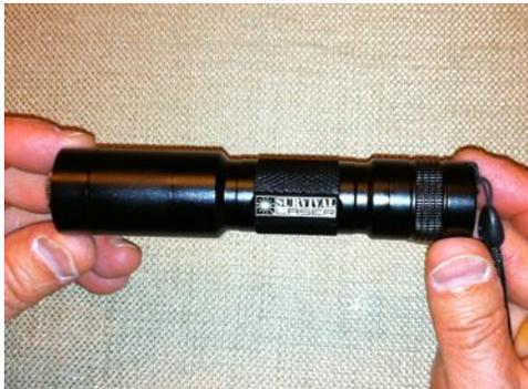
10. Point your laser in a safe direction, away from people, animals and highly flammable materials. Thread the tailcap w/switch onto the battery compartment until seated. If your laser begins functioning, press the tailcap switch to turn it off. **Important Note: Read the section about focusing on the "Laser Operation" page BEFORE using your laser.**
