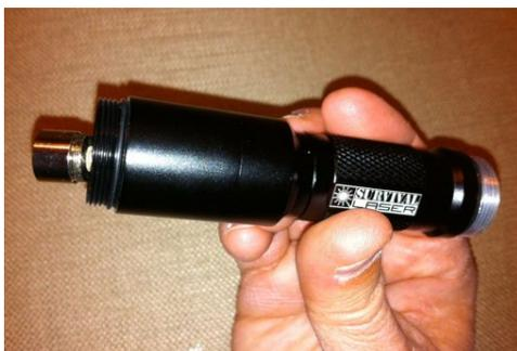
4. Carefully slide the heat sink holder over the driver assembly and thread it onto the battery compartment until fully seated. **Be careful not to twist or bend the driver leads excessively.** There will be some resistance to threading as the battery compartment o-ring is engaged into the heat sink holder during the last two threads.
