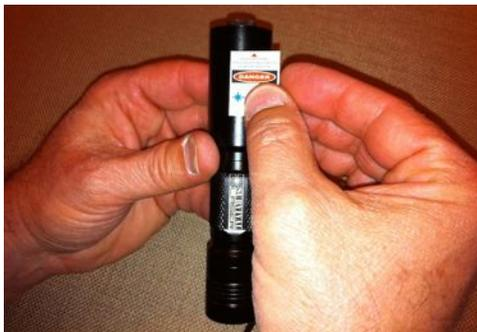
11. Fill out and apply the laser warning label to the heat sink holder, slightly overlapping the battery compartment if necessary. "Max power" is 500mW, "Wavelength" is 635nm, "Voltage" is 2.6, "Class" is 3B, "Pattern" is Point. **Note:** The red arrowhead on the label points toward the lens. Your laser is now completely assembled and ready for use.
