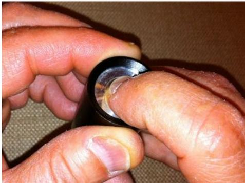
6. Place the bezel/retaining ring over the exposed end of the heat sink. Press the heat sink down with your finger and thread the retaining ring onto the heat sink holder until fully seated. **CAUTION:** Do not touch the diode inside the module with your fingers, and do not let the heat sink rotate as you tighten the bezel/retaining ring. If the heat sink rotates during tightening it could break the wires or pull them off the diode.
