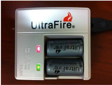
1. Plug in the charger and insert the batteries into the charger in the correct orientation shown in the battery compartments. The light on the charger will glow red until the battery is fully charged, at which time the light will glow a steady green. Once charged, remove the batteries from the charger. **WARNING: Do not** attempt to charge disposable batteries in the charger! **Note:** Charger appearance will be different that that shown.
